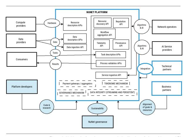
Figure 1: NuNet platform is a open-ended collection of pluggable open API, enabling providers, consumers and network operating agents to autonomously construct ad-hoc computational workflows from available components.
